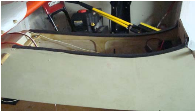
Fig 1. Fuselage contoured for Tiger 60 wing airfoil .
